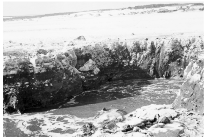
Fig. 47 Downstream of College Bridge, early morning, several hours before photo taken at location shown in Fig. 46. Snow that had fallen since previous High Water partly obscures the High Water mark. There are indications of subsidence of part of the ice wall. Photograph #359-205.
