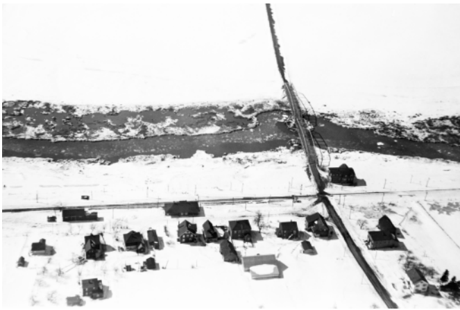
Fig. 46 Memramcook River at College Bridge, N.B., spring 1959 (see Fig. 43), shortly before noon. Note how bridge piers influence movement of ice, incoming on the tide. A natural levee, formed by ice, is commonly higher near open channels than near the banks, a condition which can lead to flooding of the more inland shore ice. Note that this and following numbered photographs were taken for the Government of Canada (DREE) by Clifford Banks, and are used with permission; this is Photograph # 359-137.
