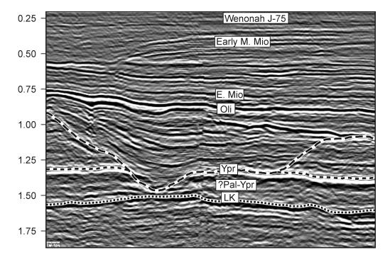
**Fig. 4** Seismic Line 83-4411a, showing erosional surface of Wenonah Canyon (\_\_\_\_), the Acadia chalk (-----), and the top of the Wyandot Formation (....). Digital seismic data courtesy of the ex-Parex Group. (Early M. Mio = early Mid Miocene; E. Mio = Early Miocene; Oli = Oligocene; Ypr = Ypresian; Pal = Paleocene; LK = Late Cretaceous.)
