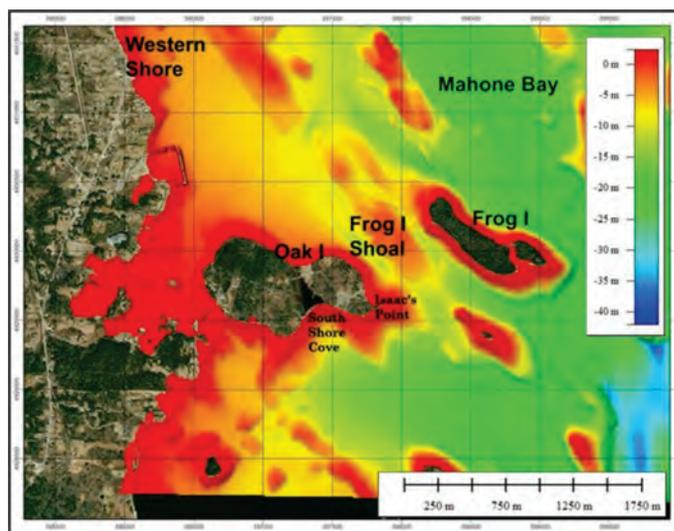
**Figure 3.** Bathymetric map of the region surrounding Oak Island, northwestern Mahone Bay. A large number of drumlin shoals are oriented northwest–southeast. Source: Canadian Hydrographic Service Non-Navigational (NONNA) Bathymetric Data, with spatial resolution of 10 metres; <https://data.chs-shc.ca/login>.
