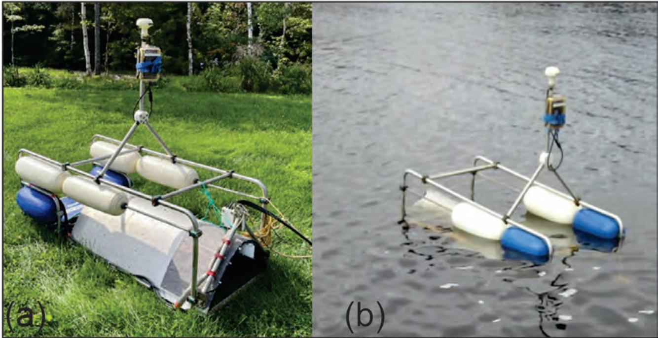
**Figure 6.** (a) Prototype Seistec profiler configured for towing reflector first. (b) Seistec profiler configured for towing boomer source first. These are the configurations used in the demonstration project described herein.
