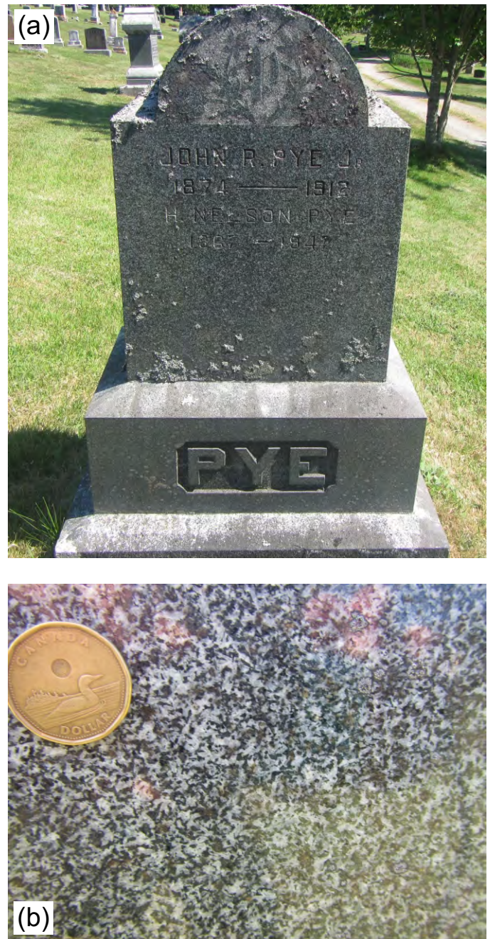
Figure 10. Monument for John Pye (1874–1912), St. Andrews Rural Cemetery (a) Glenelg porphyry (diorite) headstone (b) Close-up of equigranular texture of the stone. Loonie coin for scale.
