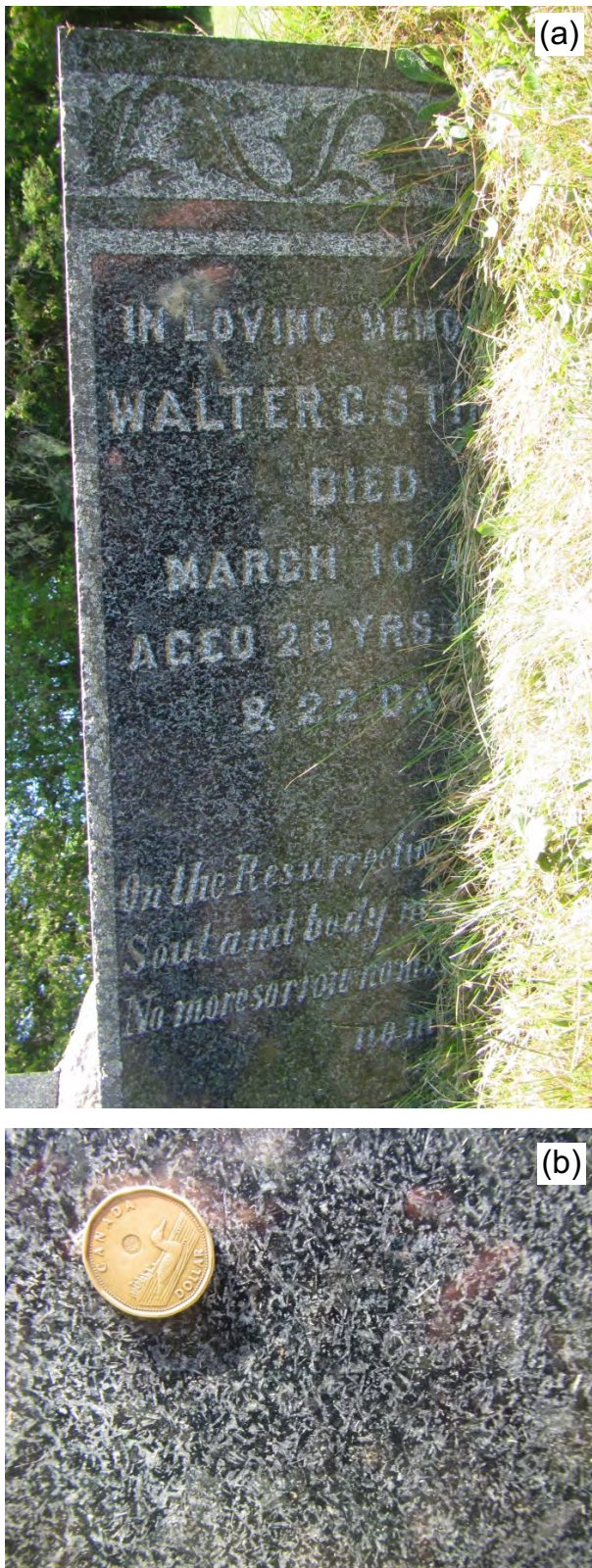
Figure 7. Monument for Walter G. Stinson (1871–1897), St. Andrews Rural Cemetery (a) Black granite (gabbro) headstone (b) Close-up of ophitic (snowflake) texture of the stone. Loonie for scale.
