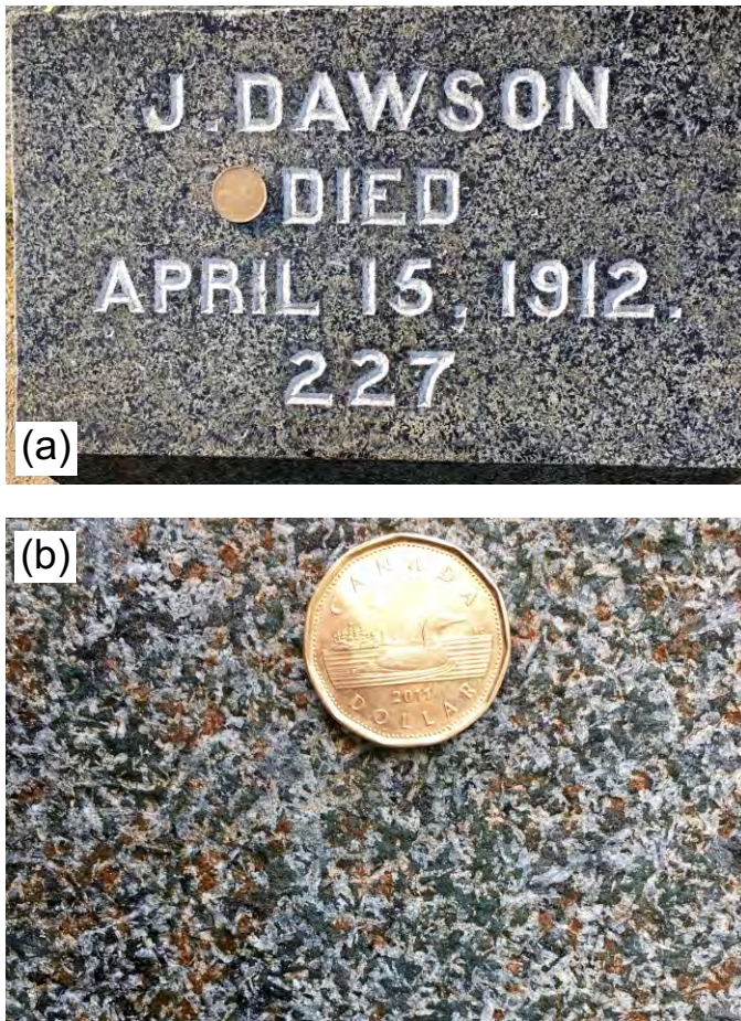
Figure 16. Monument for Joseph Dawson (1888–1912) in Fairview Lawn Cemetery, Halifax, Nova Scotia. Joseph was a member of the engineering crew on the Titanic. (a) Black granite (gabbro) headstone displaying ophitic (snowflake) texture. (b) Close-up showing abundance of reddish-brown spots likely from the alteration of olivine. Loonie coin for scale. Photographs provided by Barrie Clarke.
