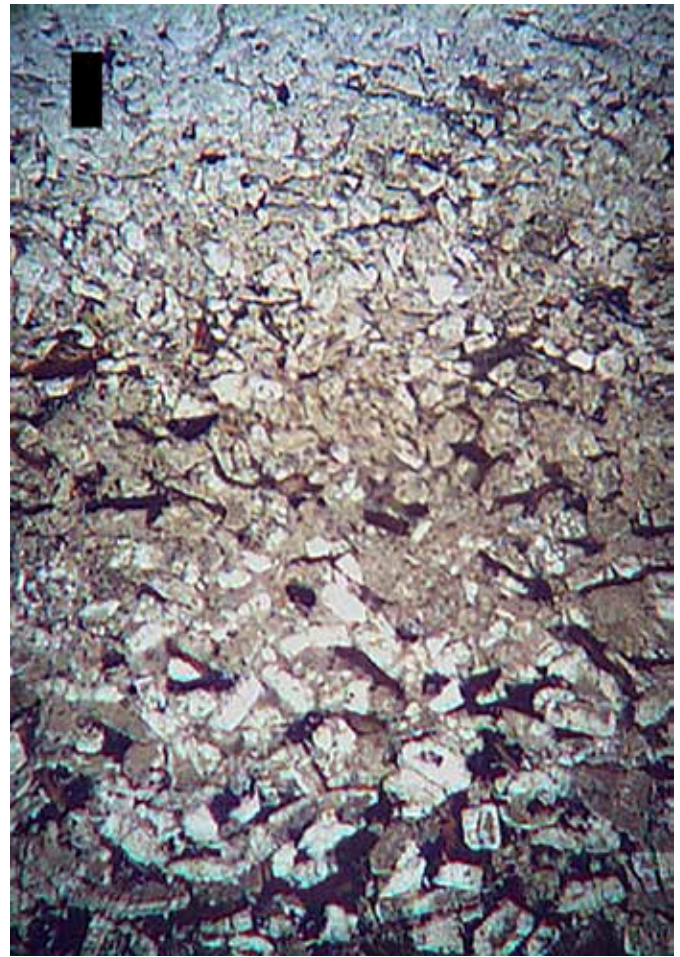
Figure 8. Photomicrograph of graded accumulation of phenocrysts at the base of tephra B. Phenocrysts are dominated by plagioclase, K-feldspar and quartz. Biotite occurs throughout but becomes more common at the top of the graded interval. Scale bar is approximately 1.0 mm.
