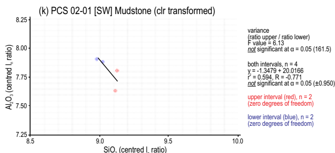
Figure 6. (previous page and below) Plots of \text{SiO}_2 vs. \text{Al}_2\text{O}_3 indicating that variances are not significant (except PCS-02-05) and correlations are mainly negative. Symbols area as in the legend for Figure 5. Abbreviations: F= variance statistic, n= number of samples analyzed, r^2 = coefficient of determination, R= correlation coefficients, and \alpha = values of significance.
