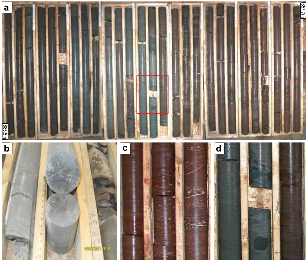
Figure 4. Images of PotashCorp core from the Penobscus area of New Brunswick. All core is 2.25 inches diameter (for scale). (a) Example of a complete core interval through the Bluish-grey Sandstone Interval, borehole 02-05. (b) Abundant coalified plant debris preserved on bedding planes (broken core slabs) in the Bluish-grey Sandstone Interval, 02-01. (c) Calcite-sealed fractures and calcareous concretions within the Upper Red Sandstone-Siltstone interval, 02-01. (d) Detail of mudstone rip-up clasts from the area shown in the red rectangle in 4A.
