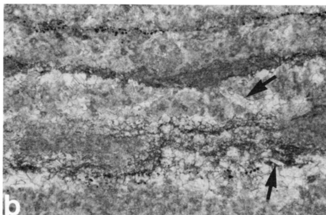
Fig. 5. Photomicrograph showing shear-related fibrous calcite (arrows). Displacement of solution seams by fibrous calcite (lower right arrow) suggest that shearing is post-chemical compaction. Plane polarized light, long axis of the picture is 1.8 mm. Sampling site #13, Port Hasting. Sample skb93-26.
