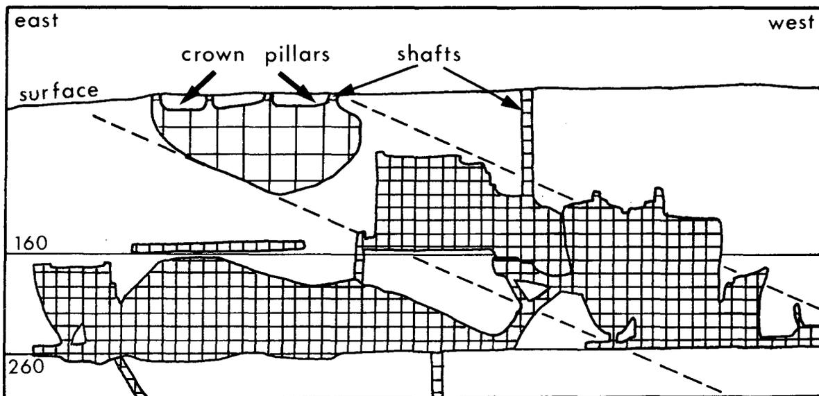
Fig. 5. Longitudinal section of mine workings on the Hewett lead as of August, 1937, taken from the assessment files of the library of the Nova Scotia Department of Natural Resources. Older, near-surface workings were accessed by multiple short shafts in the vein. More recent workings were accessed from the 49 and 79 m (160 and 260 foot) levels of the Stuart shaft. Dashed lines indicate the rake of an oreshoot within the vein.
