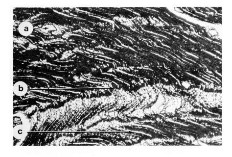
Fig. 2. Wood Specimen NO. 1. Cross section of wood in collapsed area, enlarged (210X)
