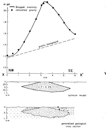
FIG. 2 An interpretation of the Golden Grove gravity high in Southern N.B. (Profile X-X')
