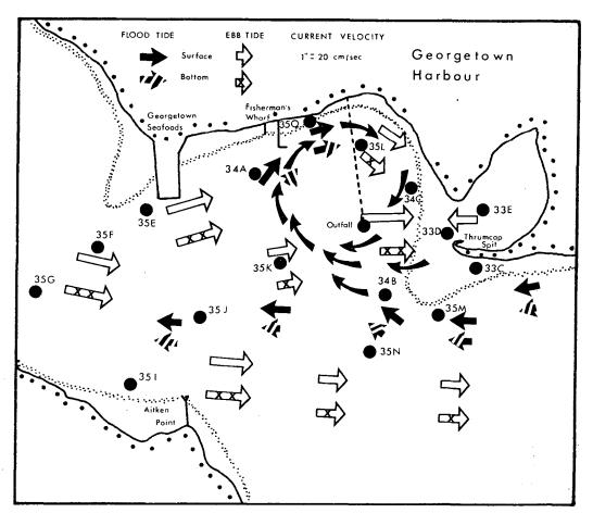
FIG. 3 Flow patterns and current velocities during flood and ebb tides in Georgetown Harbour at the mouth of the Cardigan Bay estuary. Note the clockwide gyre adjoining Thrumcap Spit and the main harbour during flood tide. Sewage and sediments are dispersed by the currents associated with this gyre.
