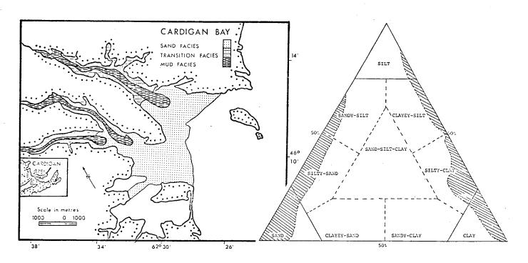
FIG. 8 Ternary plot and lateral distribution map of sediments in the Cardigan Bay estuaries. Note the distinct bimodal nature of the sediments. Fine-grained clay and silt are dominant in the rivers and adjoining wharves and outfalls; silty-sand and sand characterize the open bay.
