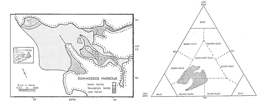
FIG. 6 Ternary plot and lateral distribution map of sediments in Summerside Harbour. Note the dominance of sand in the transition facies being reflected in the ternary diagram.
