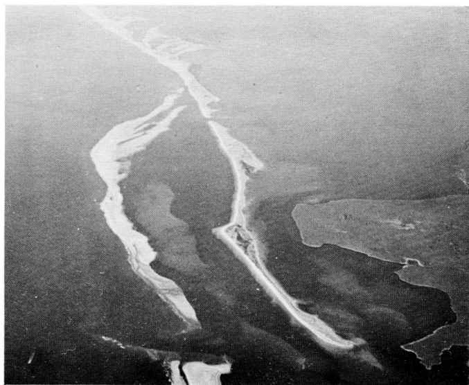
FIG. 7 Overlapping barrier islands at Neguac, Miramichi Estuary N.B. These low barriers are migrating to the south (towards the top in this photograph).
