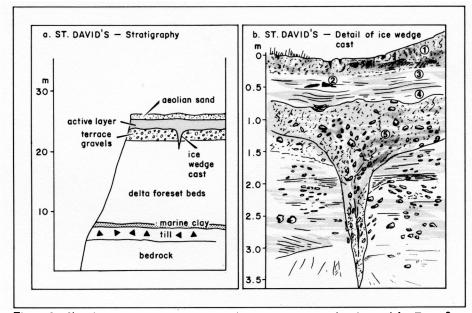
Figure 2 - Sketch of stratigraphy and ice wedge cast at St. David's. Legend for Figs. 2 and 3: 1. modern soil; 2. partyly decayed tree roots; 3. stratified aeolian fine and very fine sand; 4. structureless aeolian fine sand; 5. cryoturbate layer.
