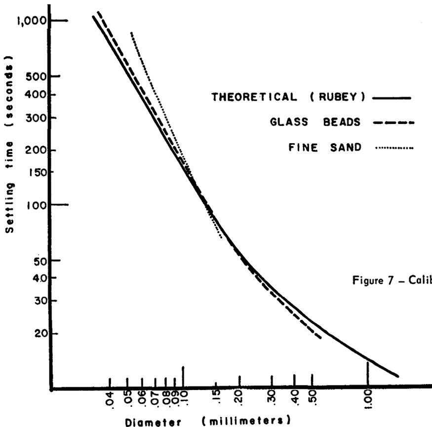
Figure 7 - Calibration curves for settling tube.
