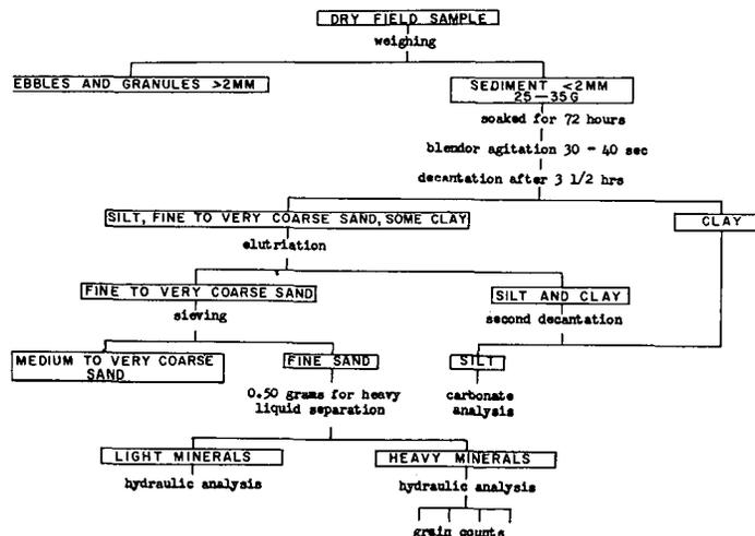
Figure 4 - Flow diagram of laboratory procedure.
