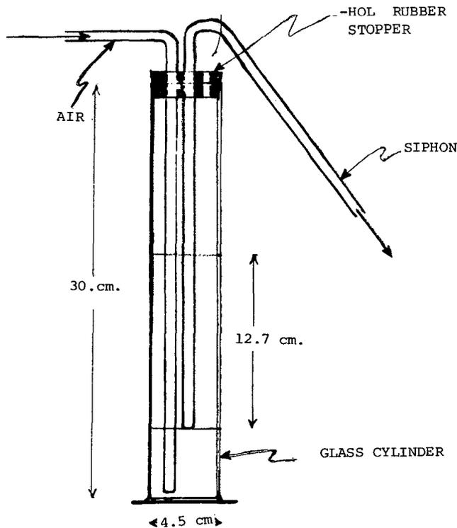
Figure 5 - Elutriation apparatus.
