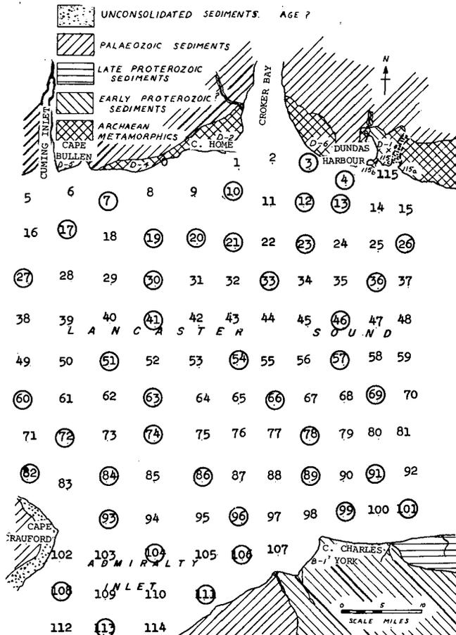
Figure 2 - Area geology and sample locations. Numbers in sound are station and bottom sample numbers. Circled numbers are samples analyzed hydraulically and mineralogically. Number and letter indicates shore sample for which thin section has been made and described. AA1 is profile line.
