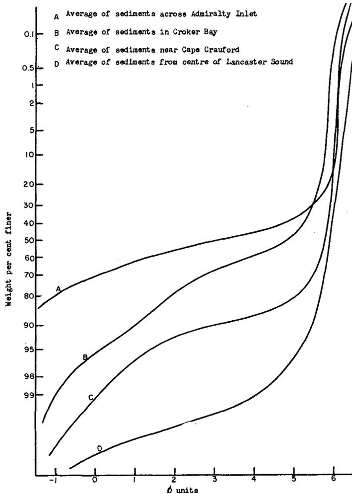
Figure 26 - Cumulative frequency distributions of sediment grades.
