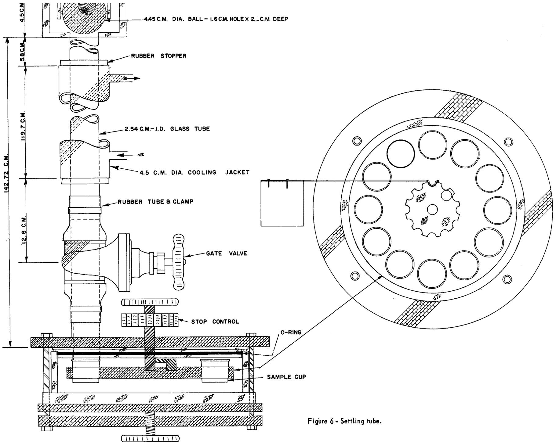
Figure 6 - Settling tube.
