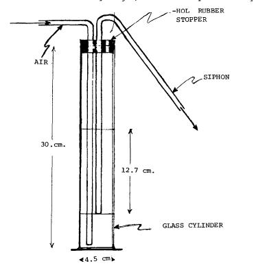
Figure 5 - Elutriation apparatus.
