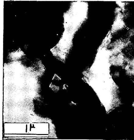
Figure 4 - High voltage transmission electron micrograph of flocculated grundite illite impregnated with polyethylene glycol. Flocculated in salt water (Na Cl 1gm/l.) x 28000.
