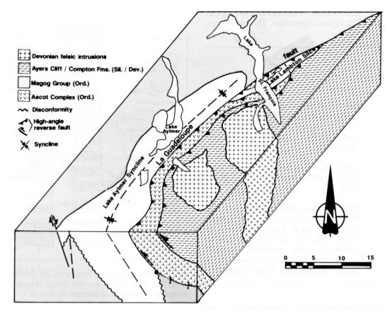
Fig. 4. Schematic block diagram illustrating the structural domains and lithotectonic units of the studied area. The Lac Aylmer and Lac Lambton formations are shown in white.
