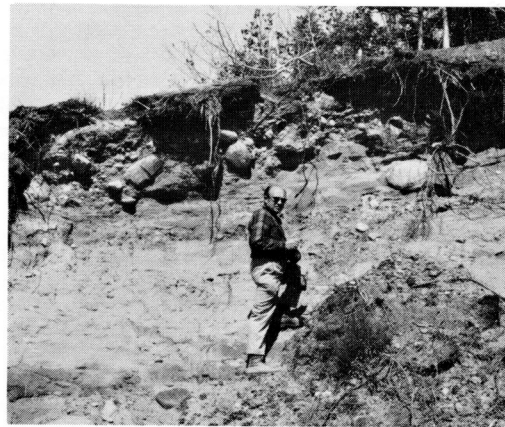
Fig. 9. La Cyr, Coffin Island. Borrow pit exposure showing bouldery mantle deposit resting on 1 metre fine medium sand, with a basal gravelly layer, overlying some 3 to 4 metres fine medium sand.
