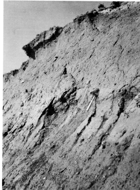
Fig. 8. Southwest coast, Amherst Island. Section shows 1 m of faintly-stratified gravelly sand passing downward into red diamicton over red sandstone. Hammer head at base of diamicton. Bedrock surface is irregular. Foreign stones are rare.
