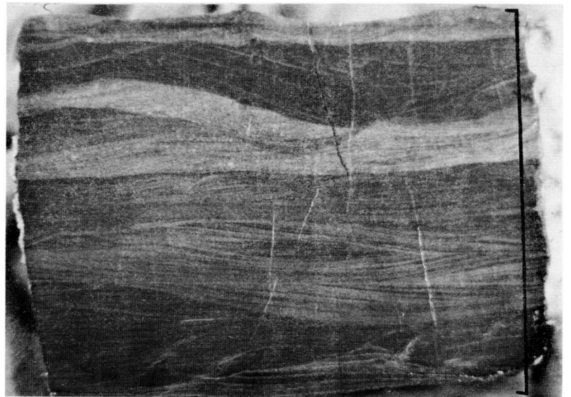
Fig. 25 Festoon cross-lamination in sandstone. The dark colour is associated with silt-rich and hematite-stained sediment. Bar represents 9.4cm.
