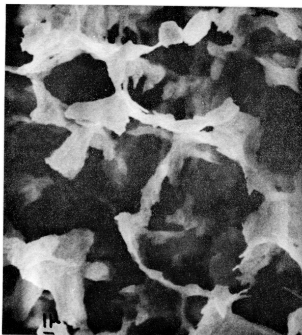
FIGURE 5 Scanning electron micrograph of freeze-dried flocculated kaolinite, x 2000.
