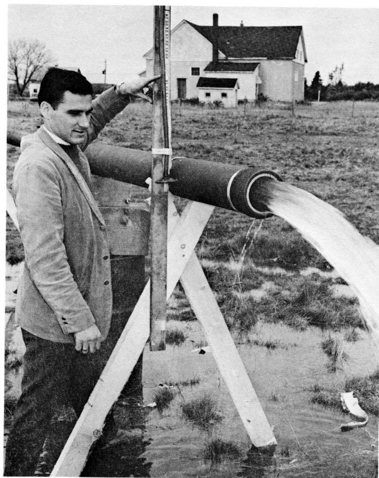
Figure 3 Recent pumping test (rate 430 imp. gallons per minute) of a sand and gravel aquifer near Truro, N.S. Aquifer is capable of producing several million gallons per day. Photo by Nova Scotia Information Branch.
