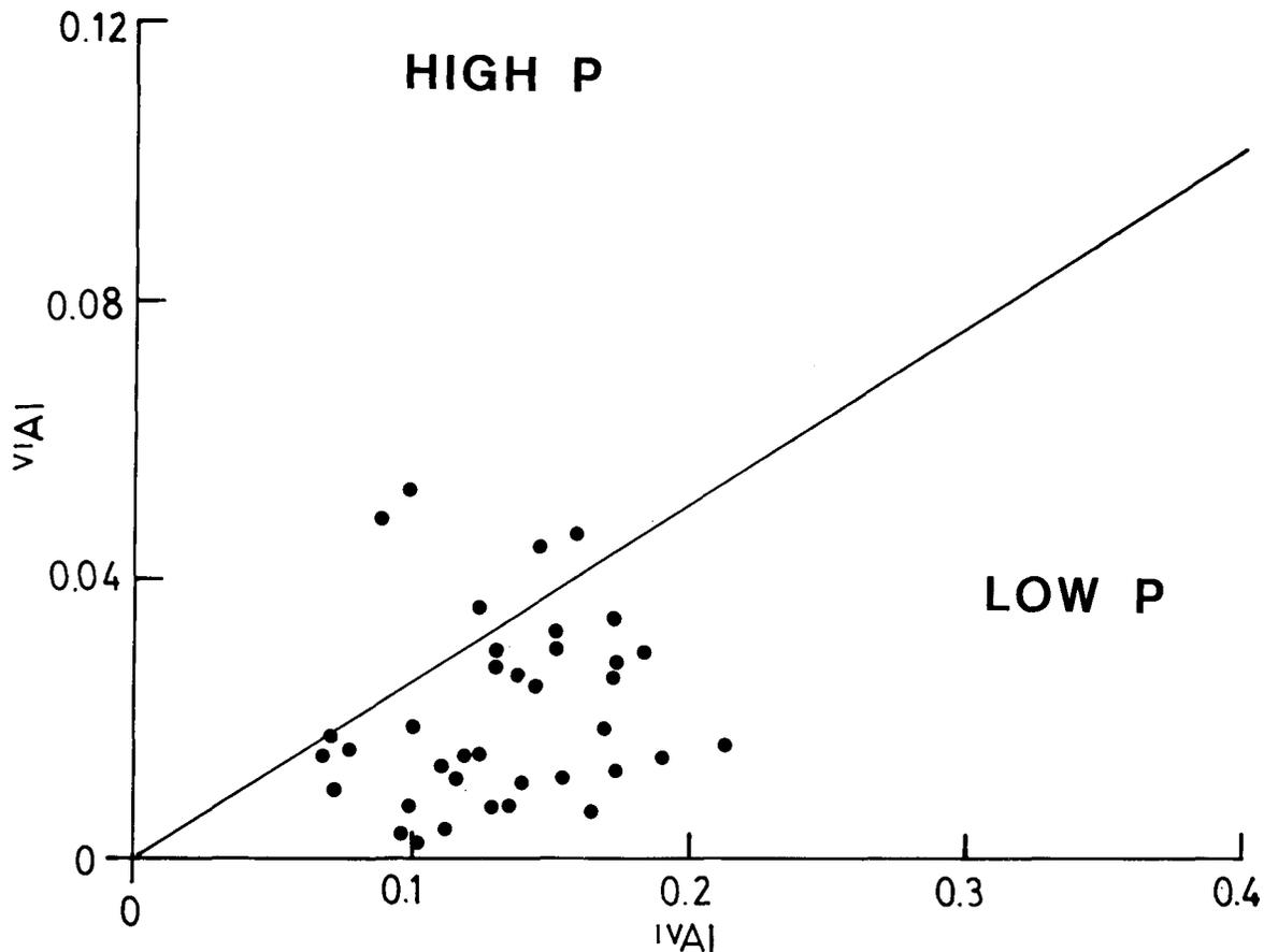
Fig. 3. Plot of  $^{26}\text{Al}$  versus  $^{24}\text{Al}$  for pyroxenes from the Folly River Formation mafic rocks. Line separates high-pressure field (upper left) from low-pressure field (lower right, after Wass, 1979).
