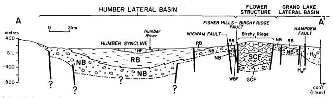
Fig. 3. Geological cross-section and topographic profile (see Figure 1 for line of section across the Deer Lake Basin) showing flower structure and lateral basins in "steers-head" profile. NB - North Brook Formation; RB - Rocky Brook Formation; HF - Humber Falls Formation; WBF - Wigwam Brook Formation; SCF - Saltwater Cove Formation; GCF - Gold Cove Formation; HoF - Howley Formation. Unornamented area below Deer Lake Basin fill represents pre-Carboniferous basement.
