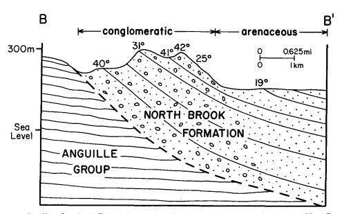
Fig. 5. Longitudinal cross-section (line of section in Fig. 1), along the Glide Lake pull-apart basin showing proximal North Brook conglomerates and more distal sandstones unconformably overlying the Anguille Group (normal faulting near the contact is also probable due to tensional stresses). North Brook sandstones continue to dip gently to the northeast (right on section), leading to a homoclinal thickness of about 7 km.
