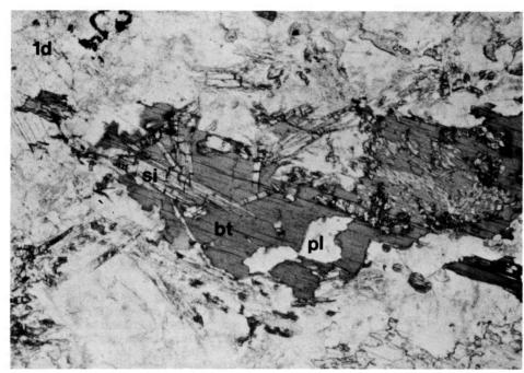
Plate ld. Large flake of secondary biotite containing abundant sillimanite (fibrolite) crystals. Note that the sillimanite is not confined to the biotite. Field of view is 0.4 mm. si: sillimanite, bi: biotite.
