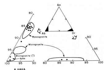
Fig. 8. Composition of feldspars from the HAHA zone (solid dots) plotted in the An-Ab-Or diagram. Data is compared to fields delineated by Kontak and Corey (in press) for several units of the BIPI suite.
