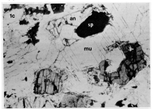
Plate 1c. Small (<1 mm) hercynite-spinel grain (isotropic) occupying core of andalusite crystal. Field of view is 0.4 mm. sp: spinel
