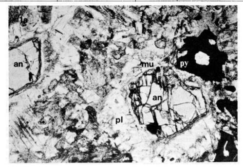
Plate la. Andalusite crystals surrounded by bleached halo composed of oligoclase ( $An_{11}$ - $An_{16}$ ). Clustered around the perimeter are masses of pinite and biotite. Field of view is 1 mm. an: andalusite, mu: muscovite, p1: plagioclase, py: pyrite.
