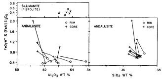
Fig. 3. Aluminosilicate mineral chemistry; note the strong (FeA1)Si<sub>2</sub>O<sub>5</sub> zonation within the andalusites.
