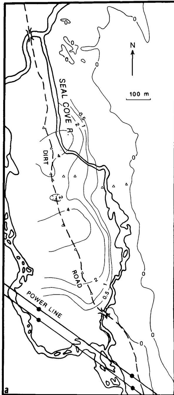
Fig. 2. a) contoured overburden thicknesses interpreted from refraction hammer seismic profiles; b) contoured overburden thicknesses interpreted from EM surveys; c) contoured granite resistivities,  $\rho_2$ . Coincident areas of low seismic velocity for the granite layer ( $V_1$  4000 m/s) indicated by solid  $\Delta$  inside 4000 m contour; d) contoured overburden thicknesses from direct probe survey; NOTE: all contours in meters; contour intervals are variable.
