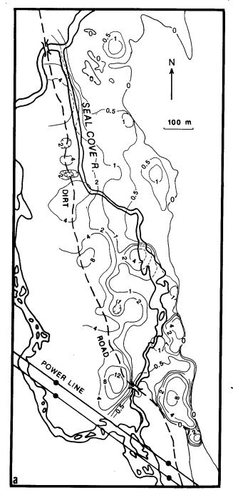
Fig. 3. a) contoured overburden thicknesses from combined data; b) contoured buried granite surface as elevations above sea level in meters. NOTE: all contours in meters; contour intervals are variable.
