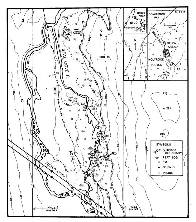
Fig. 1. The Seal Cove River valley showing topography, survey locations, bog areas and outcrop boundaries ("0" contour line); the vertical lines within the map show the borders for Figs. 2 and 3; the insets show location and geological setting of the study area; all contours in meters; north is true north for this and all other Figures.
