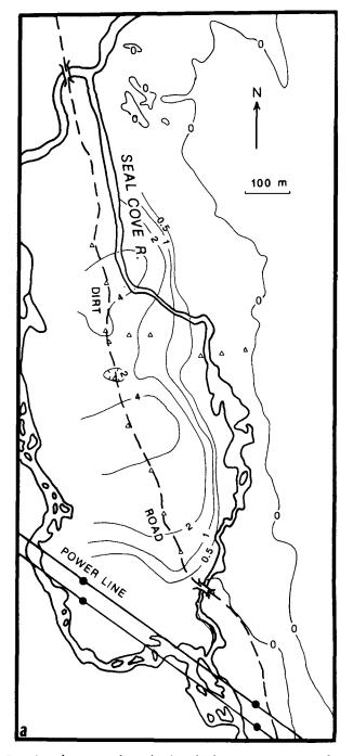
Fig. 2. a) contoured overburden thicknesses interpreted from refraction hammer seismic profiles; b) contoured overburden thicknesses interpreted from EM surveys; c) contoured granite resistivities,  $\rho_2$ . Coincident areas of low seismic velocity for the granite<sup>2</sup> layer (V1 4000 m/s) indicated by solid  $\blacktriangle$  inside 4000 m contour; d) contoured overburden thicknesses from direct probe survey; NOTE: all contours in meters; contour intervals are variable.
