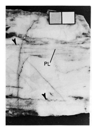
Fig. 3 - Sawn face of sample, phyllosilicate laminae indicated (PL). Note jagged structures (arrowed) which truncate phyllosilicate laminae. Sample from Harrigan Cove. Scale = 2 cm.
