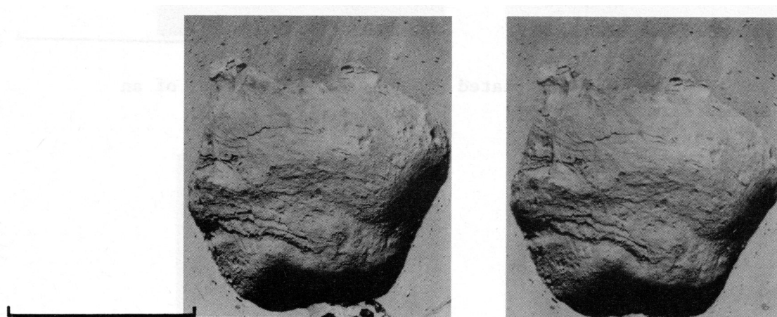
Fig. 9 - (stereopair). Well-developed, strongly asymmetrical transverse ridges on the walls of an experimental mud intrusion. Ridges are oriented perpendicular to the direction of mud intrusion.
