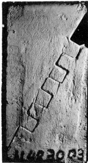
Figure 1. Unconfined test block in uniaxial compression (load applied vertically): tension fractures have developed sub-parallel to the direction of the discontinuity.
