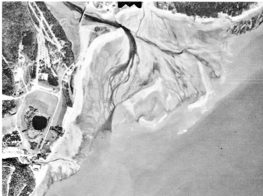
Figure 2. Alma River delta at low tide: aerial photograph, 1962. Note the changed courses for the main distributary and the side stream (Cleveland Brook); the growth of bars across the former distributary mouths, and the presence of a new inner bar. Width of area shown about 6000 feet.
