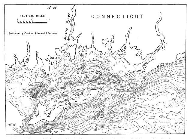
Fig. 2. Bathymetry of Fishers Island Sound. Contour interval one fathom (From U.S. Coast and Geodetic Survey No. 08084 N - 53, 1967).
