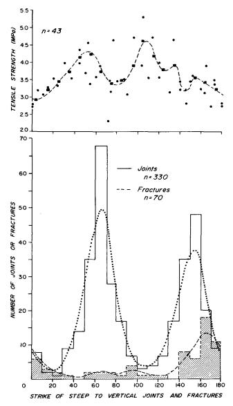
Fig. 4 - Tensile strength (above), preferred fracture orientation and joints (below) in the Perry Formation on the St. Andrews Peninsula and Minister Island, New Brunswick. Orthogonal joint sets strike 065° and 155°. Symbols as in Figure 3.
