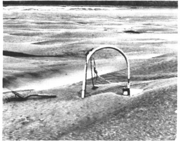
FIG. 9 Current meter in Avon River estuary near Minas Basin, Nova Scotia, buried by advancing sand waves. (Courtesy R.J. Knight, Petro Canada Ltd)
