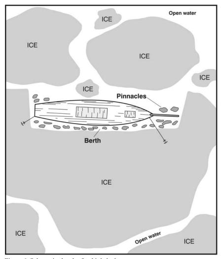
Figure 6. Schematic sketch of a ship's bed.
