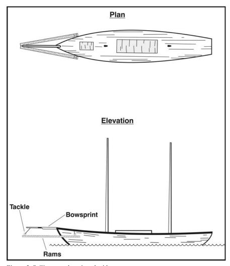
Figure 5. Sailing vessel equipped with rams.
