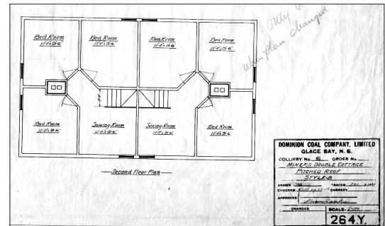
Figs. 3a (top), b (middle), c (above) “Miners Double Cottage Pitched Roof Style-B,” designed in 1905 for the Dominion Coal Company, Glace Bay, Nova Scotia. Front elevation. Scale 1/4" = 1 ft. (b) First floor plan. (c) Second floor plan. Company House Plans, 264Y. Beaton Institute, Cape Breton University.
