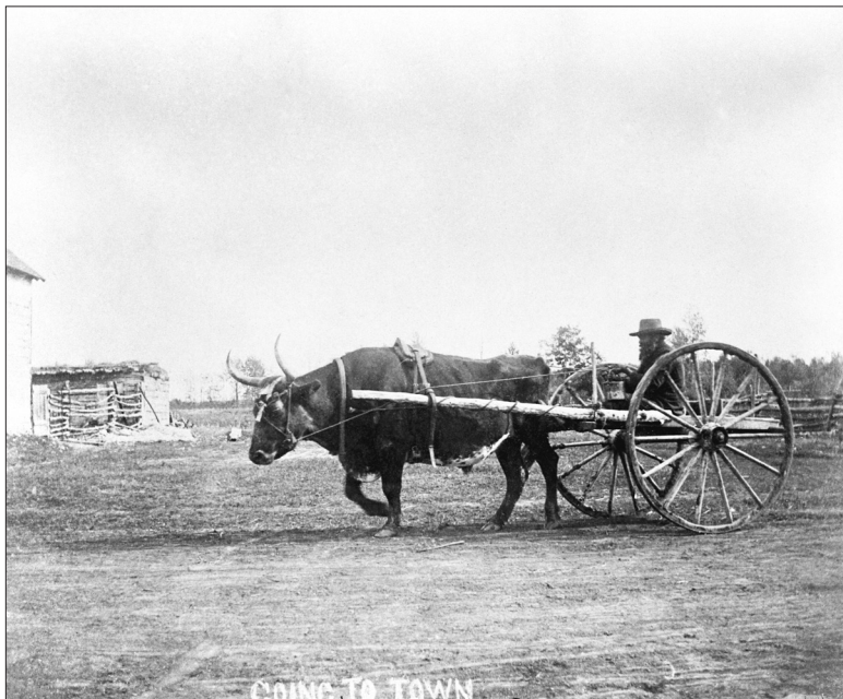
Fig. 1. Ox-drawn cart, Innisfail, Alberta, ca. 1898. Source: Glenbow Archives, NA-1709-35. Note the mouth bit and reins, and that the cart appears to be hitched only to the mid-girth and not the neck collar.
