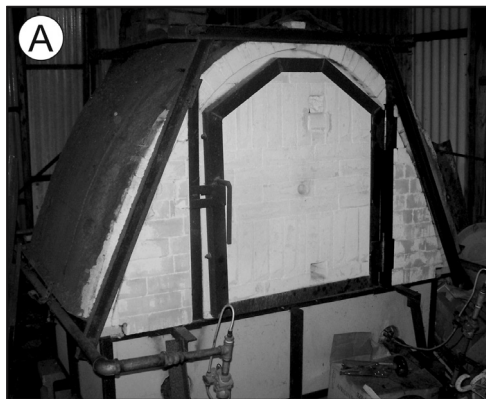
Fig. 5 Propane-fired kiln housed in a shed behind the Lorenzens' studio. A. Exterior. B. Interior. (Photos by J. Victor Owen.)
