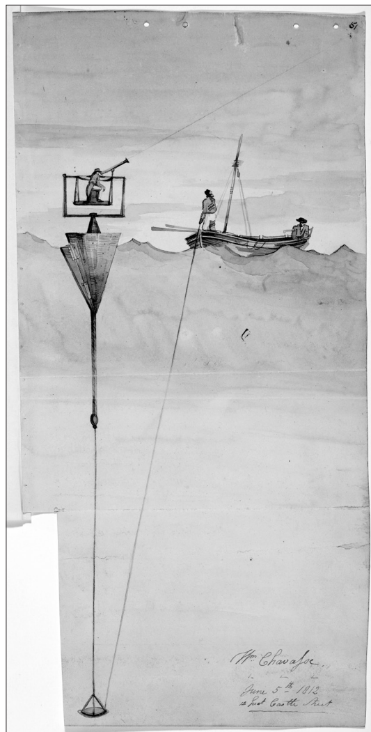
Fig. 12 This “marine chair” for steadying an astronomical observer at sea was submitted to the Board of Longitude during the early 19th century. Cambridge University Library, RGO 14/36: 51.
