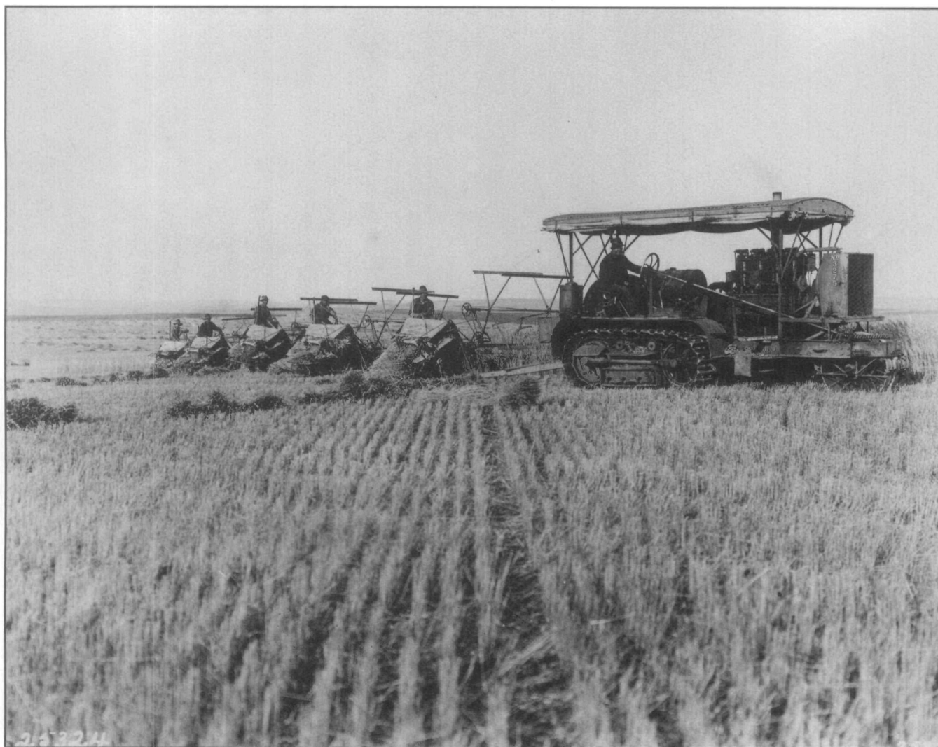
Fig. 3 Binding wheat with five binders and a Holt Caterpillar tractor, Goose Lake Line, Saskatchewan, ca 1920 (CSTM/CN Collection 25324)
