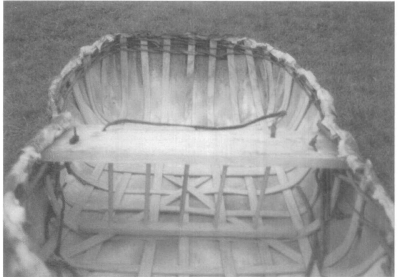
▲ Fig. 8 The coracle with its skin sewn to the basketry gunnel.
