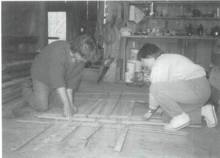
▲ Fig. 2 Traverse laths interwoven with the longitudinal laths. The first three are doubled at the bow.
