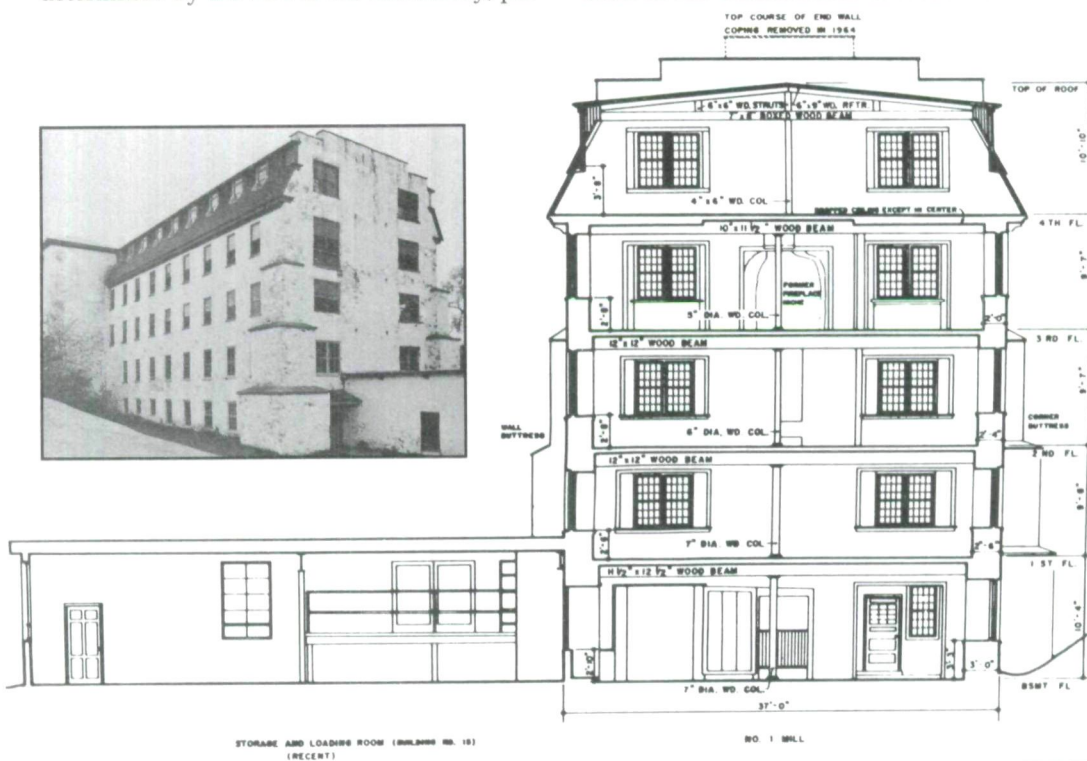
Fig. 1 The Allendale mill, Centerdale, R.I. The main block, built in 1822, is the oldest known example of a slow-burning mill. (Source: New England Textile Mill Survey [Washington, D.C.: Historic American Engineering Record, National Parks Service, 1971] p. 141)
