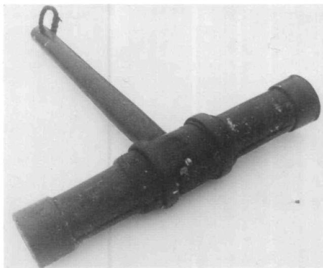
Fig. 1. Caulking mallet originally owned by William Heans (1831-1912) and used during the construction of the yacht *Canada*. (Courtesy: Howard F. Heans.)
