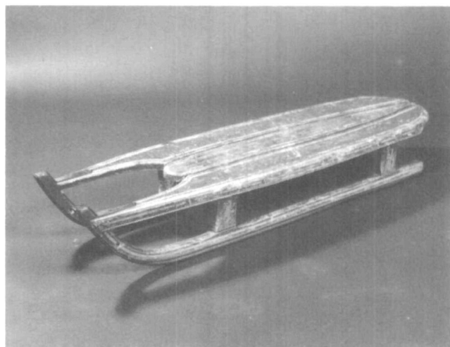
Fig. 3. Pine sled with elm runners reinforced with iron bands, c. 1860. Signed on the bottom in black crayon: "C.M. Faulkenham/Lunenburg, N.S." It is likely the work of a craft workshop, making sleds for sale to customers. Later factory-made versions were advertised by the T. Eaton Co., Toronto, in their 1901 catalogue, at prices from 20¢ to 65¢ each. Ht. 21 cm. (Cat. no. 984.88.1; neg. no. 85CAN65.)
