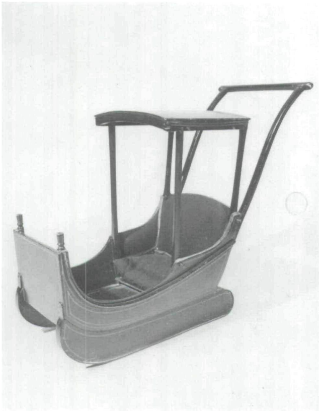
Fig. 4. Child's sleigh with original black paint and thin red decorative lines. The seat is upholstered in black wool plush edged with black braid. This sleigh was made in Quebec province about 1860, by a craftsman specializing in carriages and sleighs. This sleigh would likely belong to a child whose parents owned a full-size sleigh for their own transportation. Ht: 90 cm. (Cat. no. 972.429.1; neg. no. 78CAN276.)
