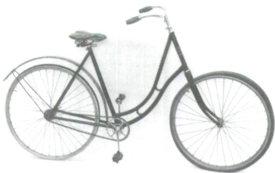
Fig. 3. Massey-Harris Model C bicycle, Massey-Harris Company Limited, Toronto, 1898. A ladies' drop frame bicycle, fitted with Dunlop Detachable Tires made in Toronto. (Photo: N.M.S.T., cat. no. 830366.)
