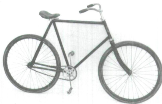
Fig. 4. Berlin bicycle, Arthur Pequegnat, Berlin, Ontario, ca. 1897. A men's diamond frame bicycle, also with Toronto-made Dunlop Detachable Tires. (Photo: N.M.S.T., cat. no. S273.)
