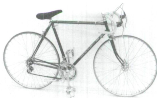
Fig. 5. Tour du Canada bicycle, CCM, Toronto, ca. 1975. A men's ten-speed model produced by the now dissolved Canadian bicycle manufacturing giant. The Tour du Canada included Campagnolo components, a 3ttt Record handlebar, an Italian-made saddle, and Universal brake components. (Photo: N.M.S.T., cat. no. 750686.)
