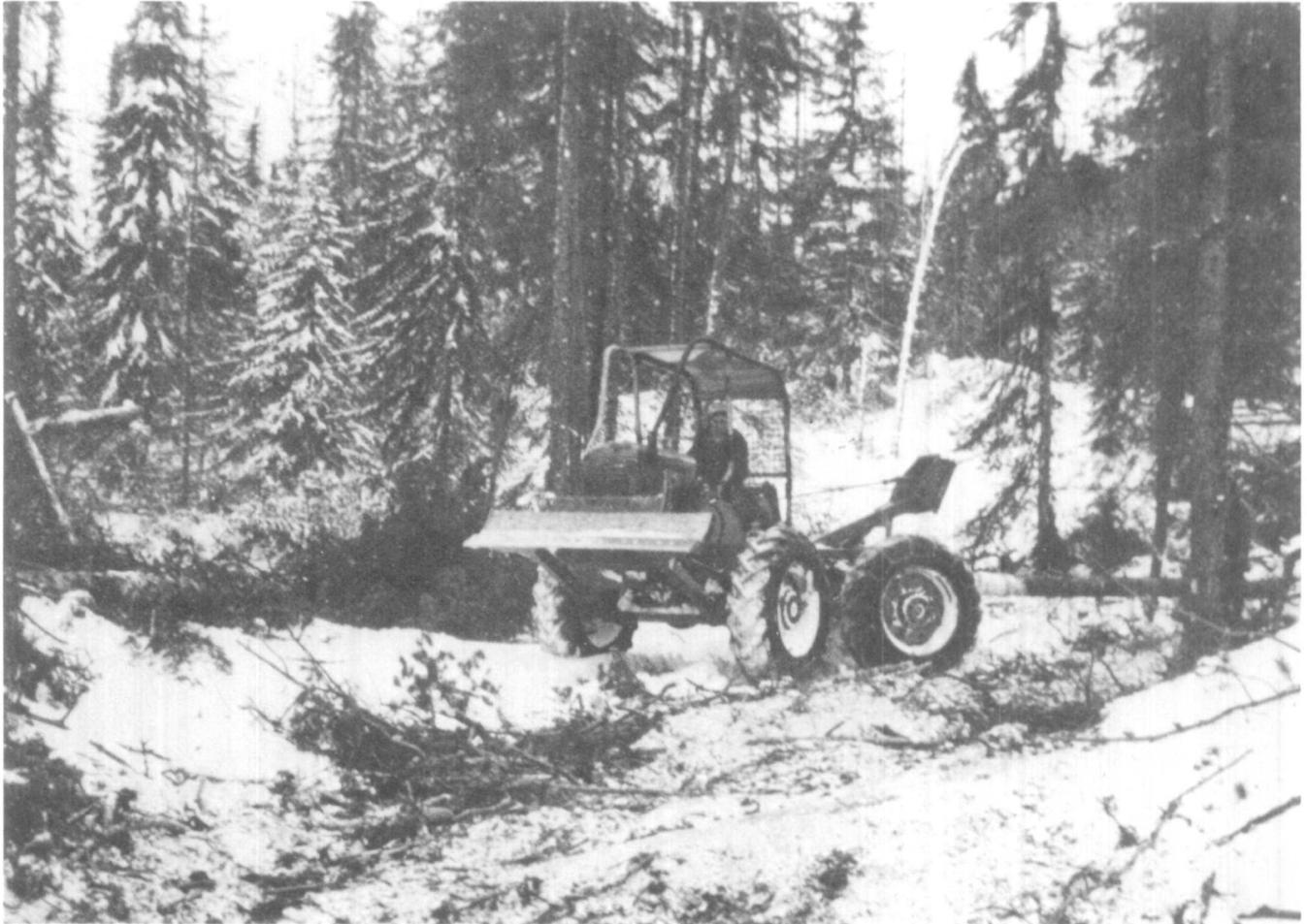
Fig. 9. Skidding with a diesel-powered articulated skidder on the limits of Dubreuil Brothers of Dubreuilville, Ontario, January 1964. (Photo: University of Toronto Archives, A73-0025, Logging Report by G.A. Bull and R.M. Rauter.)
