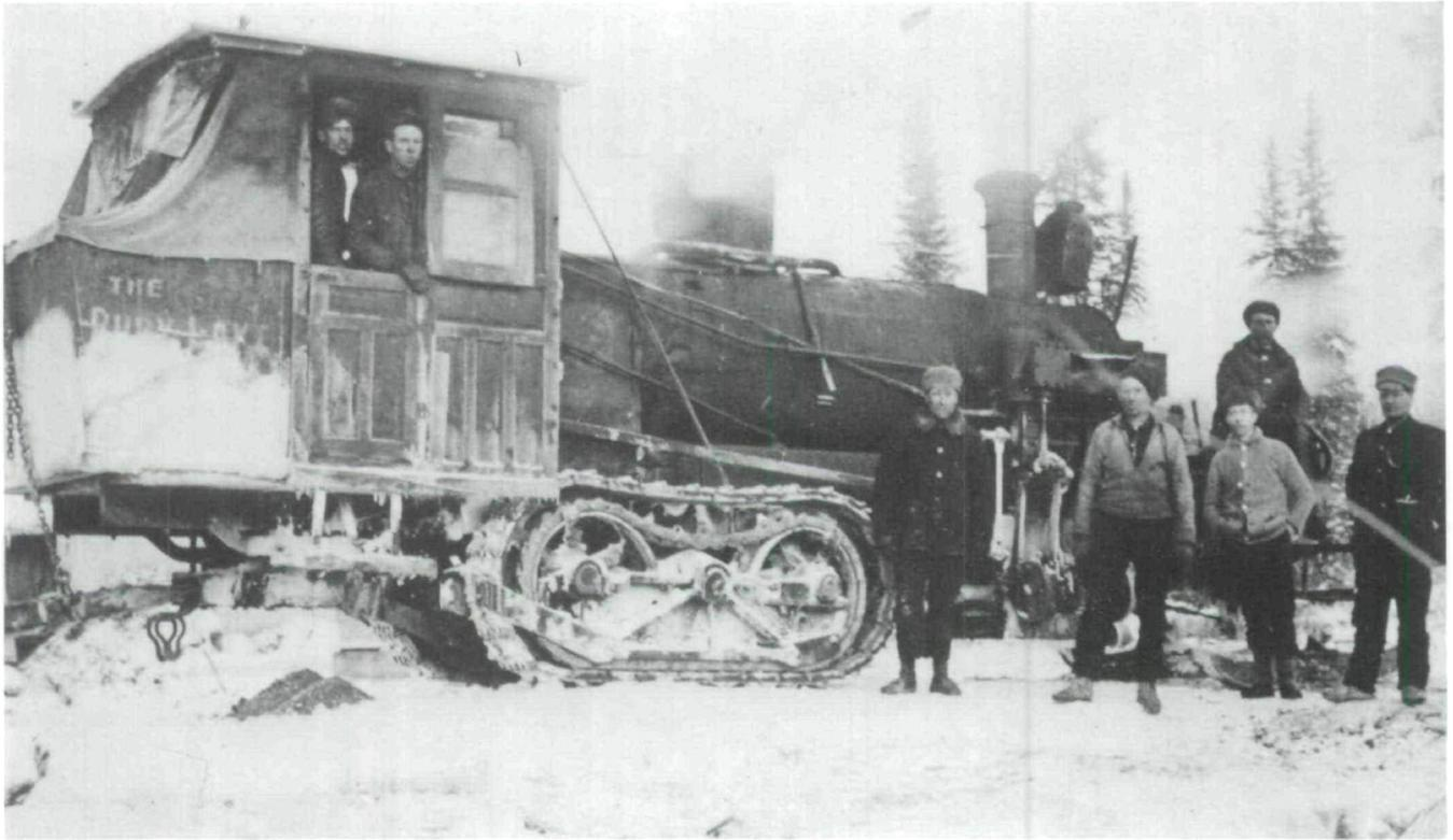
Fig. 4. Hauling crew with a Lombard Steam Log Hauler of the type sometimes used in flatter areas of northern Ontario during the first quarter of the twentieth century. (Photo: University of Toronto Archives, A73-0025, 008(15).)
