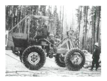
Fig. 8. Skidding pulpwood using a gasoline-powered, four-wheel drive Blue Ox skidder on the limits of K.V.P. Company, Ltd., near Espanola, Ontario, 1959. (Photo: University of Toronto Archives, A73-0025, Logging Report by R.T. Bragg and E.G. Osler, 1959.)
