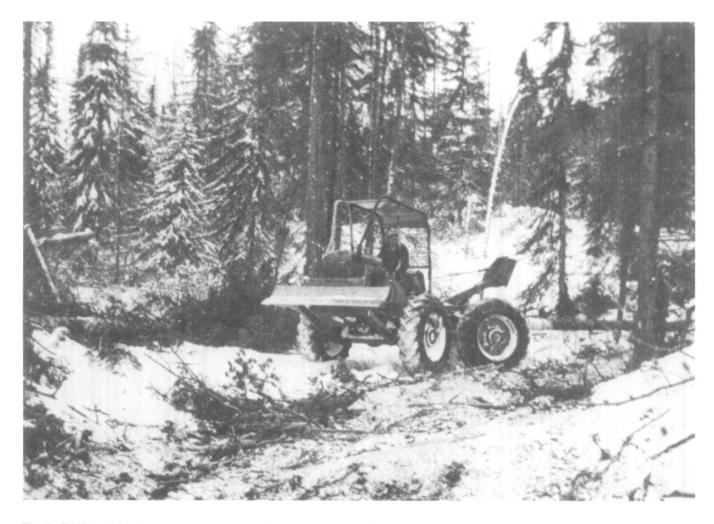
Fig. 9. Skidding with a diesel-powered articulated skidder on the limits of Dubreuil Brothers of Dubreuilville, Ontario, January 1964. (Photo: University of Toronto Archives, A73-0025, Logging Report by G.A. Bull and R.M. Rauter.)
