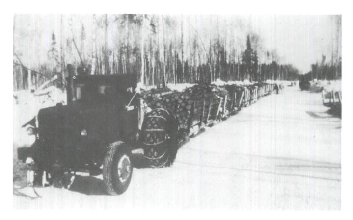
Fig. 5. Euclid 200-horsepower diesel truck pulling ten sleighs loaded with eight-foot pulpwood at Nipigon Lake Timber Company Camp 71, near Kowash, Ontario, 1948. (Photo: University of Toronto Archives, A73-0025, Logging Report by W.E. Cuff, 1948.)
