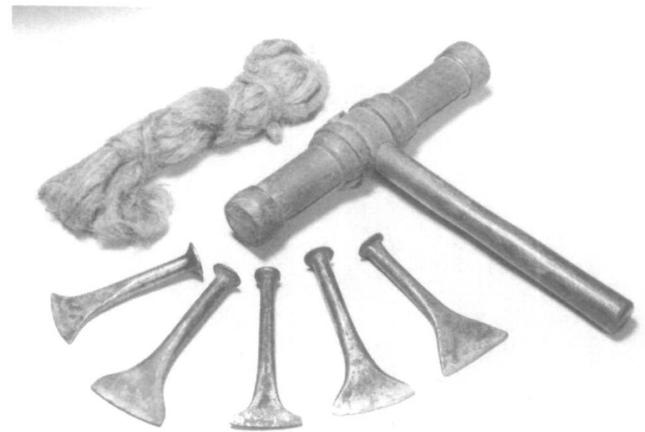
Fig. 4. Caulking hammer, irons and oakum used by ship carpenters or caulkers to make the joints of the outer planking on a ship's hull water-tight. Because a large percentage of Canadian ships were built to transport timber to Great Britain, shipbuilding and the timber trade were closely interrelated. (Photo: NMC, AC 16, 77-13.)
