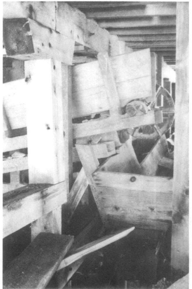
Fig. 5. Sawdust chain and troughs. (Photo: Project photograph, detail.)
