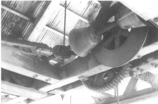
Fig. 3. Log turning winch and reversing clutch. (Photo: Project photograph, detail.)
