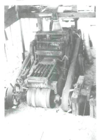
Fig. 7. Tower edger, 48", moveable blades. (Photo: Project photograph, detail.)
