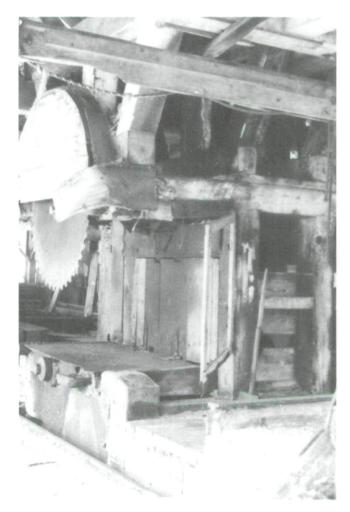
Fig. 2. Headsaw and husk, lower blade absent. Most of the machinery at Georgetown was taken to Brown's Mill before the 1978 fire. (Photo: Project photograph, detail.)
