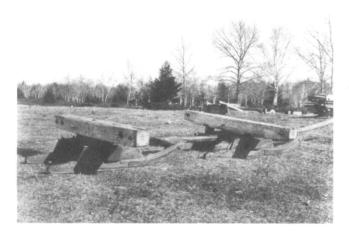
Fig. 8. A one-beam sleigh used for hauling sawlogs, ca. 1880s. (Photo: PAC, neg. no. C-30531.)
